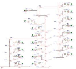
Fig. 2. Modelling of feeder network in ETAP
